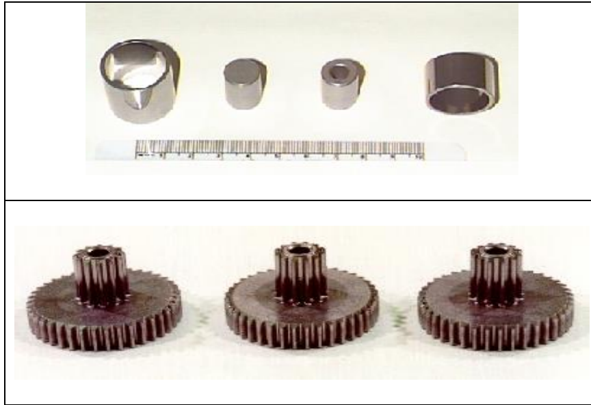
Microwave sintered commercial powder metal parts by Microwave Processing and Engineering Center of The Pennsylvania State University, USA.
